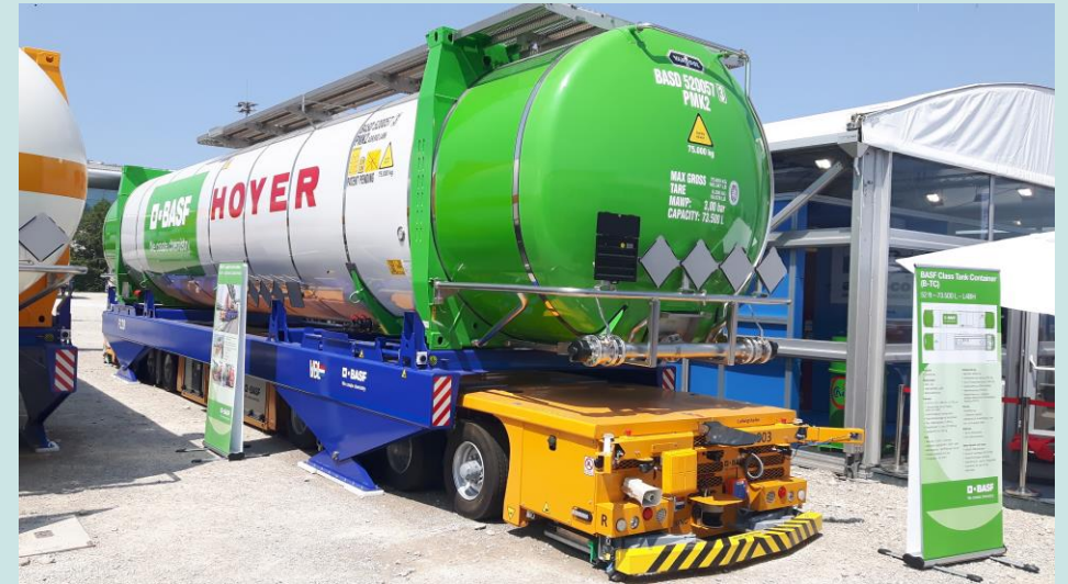
Exemplary illustration of an Underride AGV with tank container of the company VDL Steelweld
