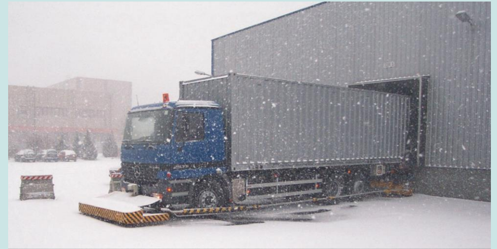
Exemplary illustration of an automatic truck in outdoor operation under difficult weather conditions
